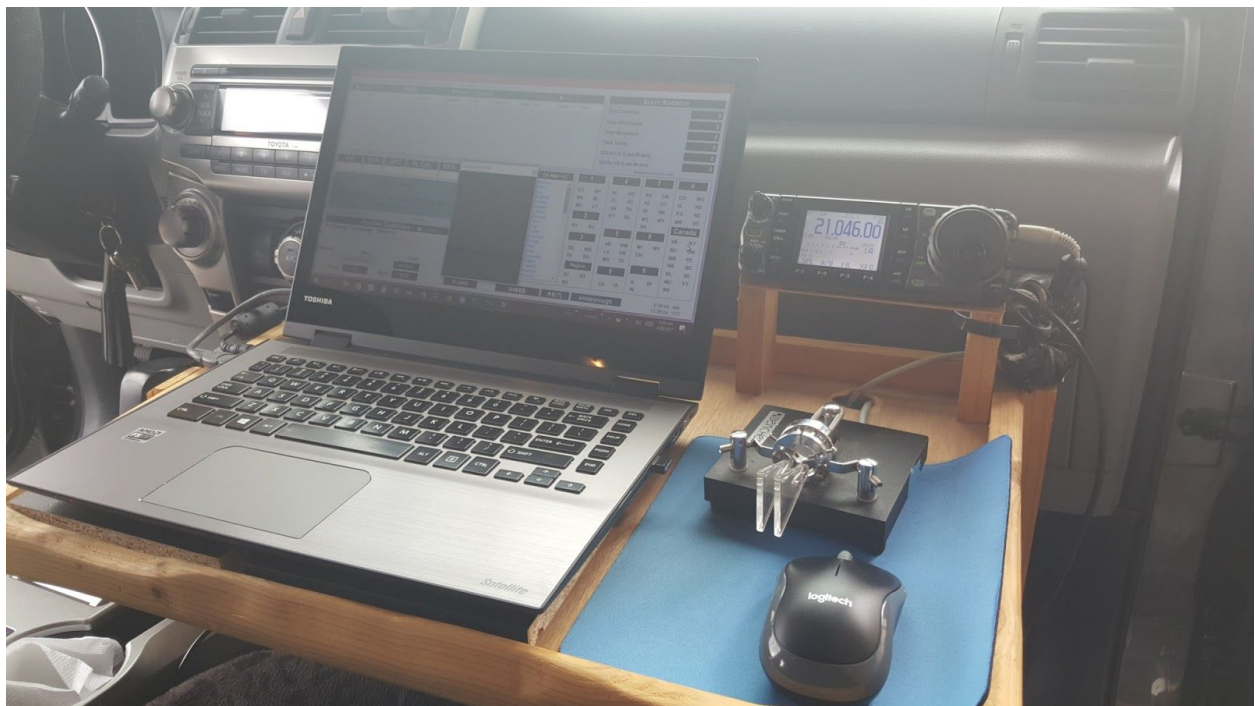
The N4EEB/m operating position - Toshiba laptop running N3FJP, Bencher BY1, and IC7000. Notice the large ferrite donut to prevent unwanted RF intrusion on the CW keyer lines
