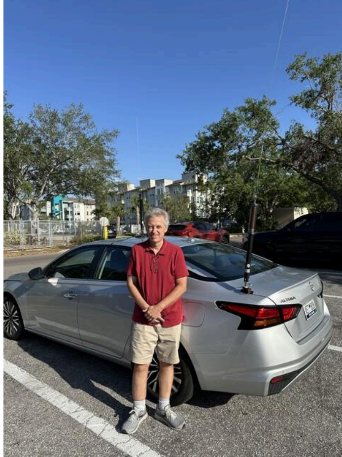
K1TO in front of the Silver Bullet; a rented 2024 Nissan Altima that housed N4TO/m. The antennas were a Tarheel Designs Little Pro HP (on the trunk lip) for 40m and a Tarheel Designs Little Pro on a magmount on the roof for 20m/15m/10m.
